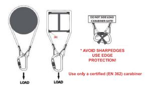
The direction of anchor device is vertical. The minimum static strength of anchor device is 12kN
